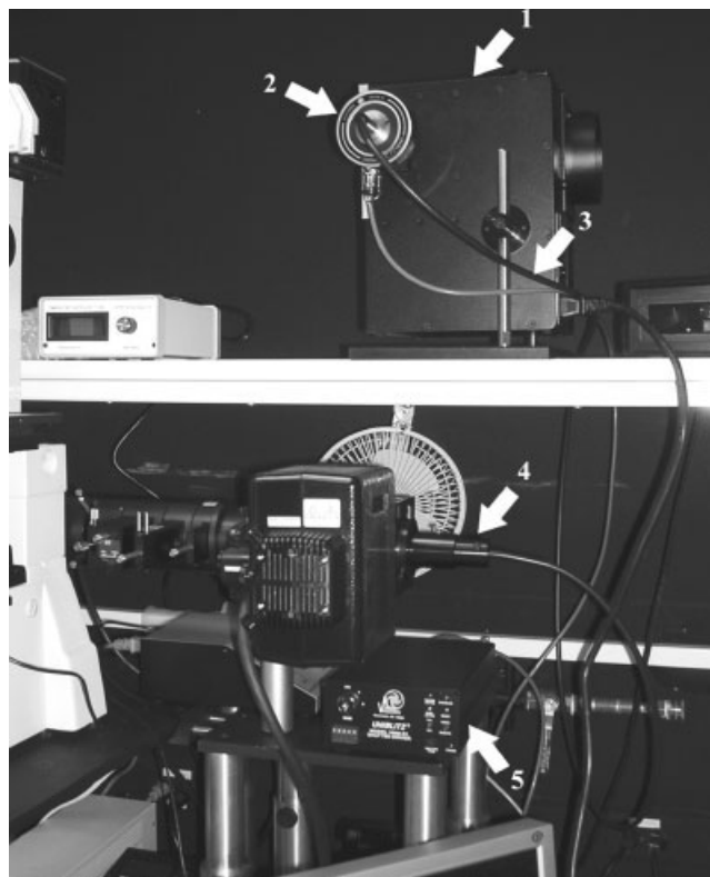
Fig. 9. Apparatus for rapid shuttering of a xenon light source. The components are numbered as follows: (1) Sutter lamp, (2) Uniblitz high speed laser shutter, (3) optical pipe, (4) microscope adapter, and (5) Uniblitz shutter control system. This system can be rapidly opened and closed to minimize sample photobleaching.
