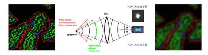
The image is the sum of all the PSFs, each centered at, and scaled in intensity, according to the corresponding point source in the sample. This is true for every image, however complex. The object convolved with the PSF forms the image, hence knowing the PSF by calculation or measurement allows a good approximation of the original object.
