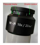
Where a microscope of either type is fitted with one or more eyepieces with built-in focusing adjustments for a photographic frame or a graticule, these should ideally be used in eyepiece tubes of adjustable length, and should be set before step 4. is carried out. For correct adjustment, microscopes having eyepiece tubes of fixed length should always be fitted with a pair of eyepieces with focusing adjustments.
