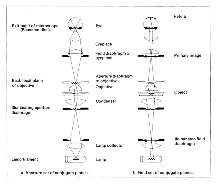
**Fig. 1**. Ray paths of the transmitted-light microscope showing (a) the *aperture* set and (b) the *field* set of conjugate planes. From the RMS Dictionary of Light Microscopy.
