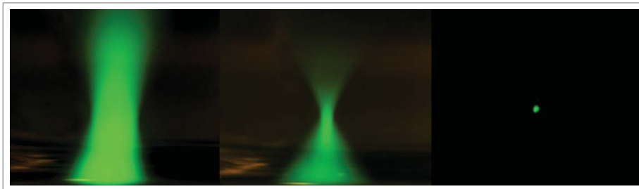
Figure 2. Distribution of fluorescein fluorescence (green) as viewed in the x-z plane, on inverted microscope, focused with 20 X objective lens 0.75NA. (A) Wide-field microscopy (WFM) mercury source and filter cube excitation. (B) Confocal scanning microscopy (CLSM), 488 nm laser excitation, and (C) two-photon (2P) excitation using femtosecond pulses of 850-nm light.
