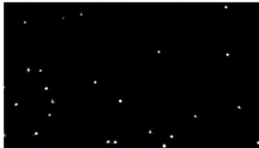
Fig.8. Lightguide-based TIRF,100X, NA 1.0 water-imm.objective. 1-um fluorescent beads.
