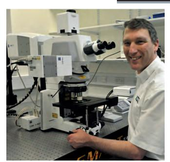
Jeremy Sanderson pictured with modern 21st century twophoton microscope with laser-scanning confocal capability. A modern research microscope such as this is multi-functional with integrated software control for consistency, reproducibility and ease-of-use. Prices vary according to the specification ordered, but can range between £100-500k
