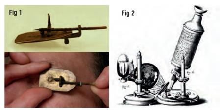
The early microscopes of Leeuwenhoek and Hooke. Many of the components found on a modern microscope (light, condenser, objective, bodytube, eyepiece) can be seen on Hooke's microscope
