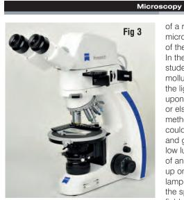
A modern entry-level polarising microscope with digital integral camera. This equates broadly with Hooke's compound microscope. The lighting is now integral within the base of the stand. The microscope can be used both in reflected-light mode (as for Hooke's microscope) or in transmitted-light mode
