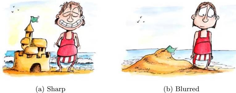
Figure 15.1: Schematic diagram showing the effects of blur. Think of the sand as photons, and the height of the sandcastle as the intensity values of pixels (a greater height indicates more photons, and thus a brighter pixel). The ideal data would be sharp and could contain fine details (a), but after blurring it is not only harder to discriminate details, but intensities in the brighter regions have been reduced and sizes increased (b). If we then wish to determine the size or height of one of the sandcastle's towers, for example, we need to remember that any results we get by measuring (b) will differ from those we would have got if we could have measured (a) itself. Note, however, that approximately the same amount of signal (sand or photons) is present in both cases – only its arrangement is different.
